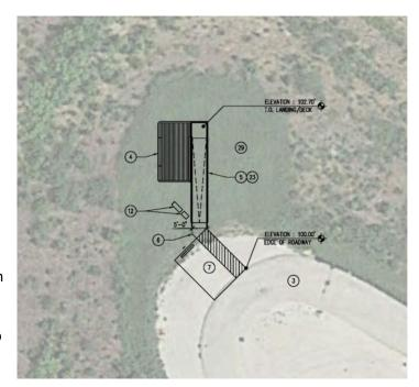
**Construction Needed**: Construct a new ADA compliant platform approximately 10' x 20' constructed of composite material. Construct a new ADA parking space and accessible sidewalk.
